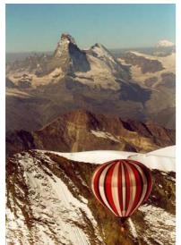
of 4 essential parts: envelope, basket, burner and gas cylinders. The envelope is made of lightweight, airtight nylon with special coating. The basket is wattled of willow, just like 200 years ago. The air inside the envelope is heated with a powerful but quite silent gas burner. The gas (propane) is carried inside the basket in steel cylinders. Modern balloons can lift between 1 and 20 passengers.
